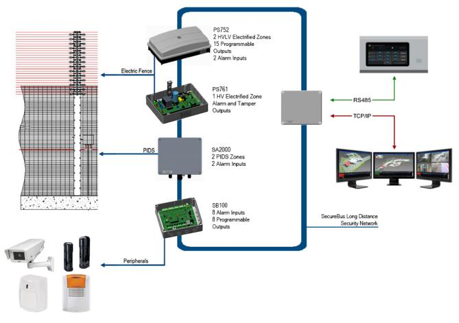
SecureBus is a communications network system developed by Harper Chalice. This network is designed to manage multiple security devices across a site and monitor alarm sensors. Designed with security in mind, the network provides robust communications with fault detection and tolerance.
